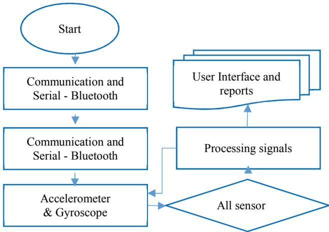
Fig. 3. Flow diagram of signal processing of biosensors.
