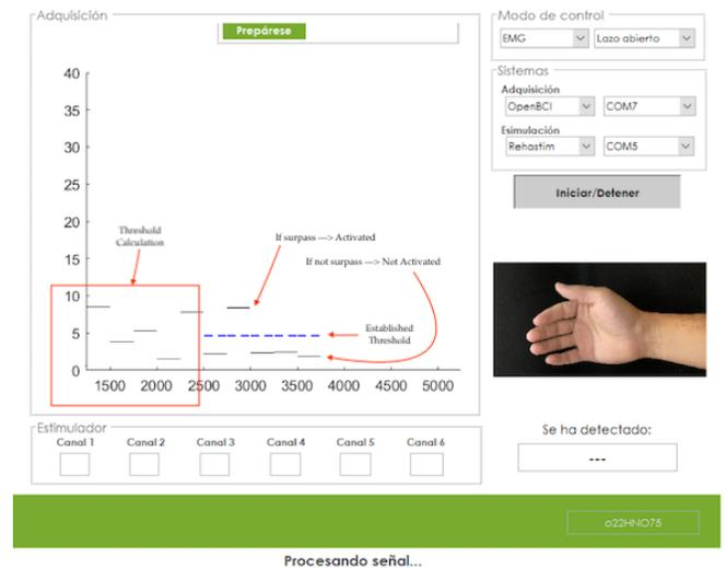
Fig. 6. ON/OFF Switch Control example. Threshold establishment and switch activation.
