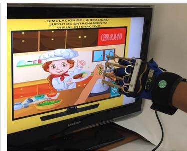
Fig. 4. The Glove Smart Hybrid system and the task-specific games of this system.
