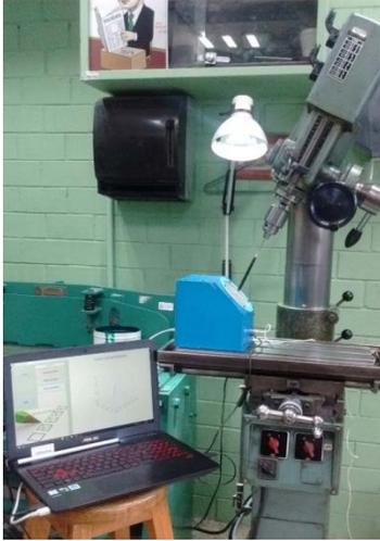
Fig. 2. Calibration of the training module, with the milling machine the ideal path of the instruments was determined.
