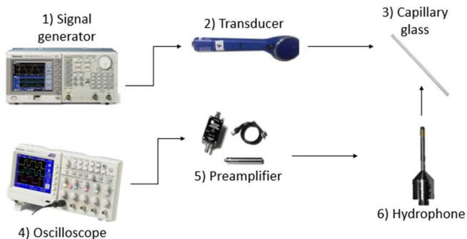
Fig. 2. Experimental setup. The hydrophone was inserted into the upper end of the glass tube, and the transducer was radiating from the bottom part of the tube.
