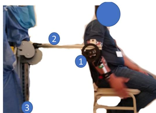
Fig. 1. Experimental Setup. 1) Deflection pulley. 2) Deflection pulley, pulley machine connection bar. 3) Pulley machine.
