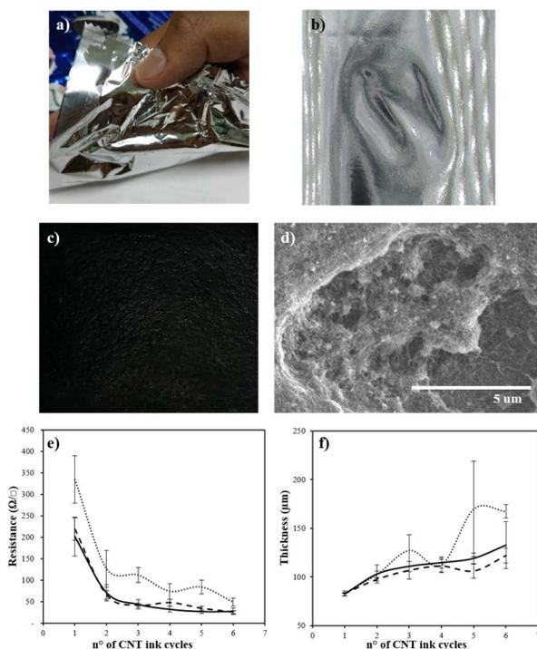
Fig. 1. (a) Recycled MPS from snack packages. (b) Conversion of MPS into a conductive MPS (c); (c) SEM micrograph of MPS painted with CNT-ink, (d) electrical resistance and (e) thickness of the MPS as a function of the numbers of cycles of CNT-ink at 80 °C (dashed line), 100 °C (solid line) and 120 °C (dotted line).
