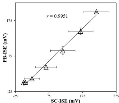
Fig. 4. EMF plot comparing the values obtained for a single calibration curve using the PB-ISE and SC-ISE for different potassium concentrations.
