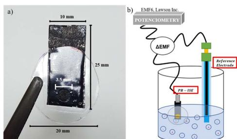
Fig. 2. (a) The final dimensions of the PB-ISE to use in (b) a potentiometric cell using a reference electrode and the final PB-ISE.
