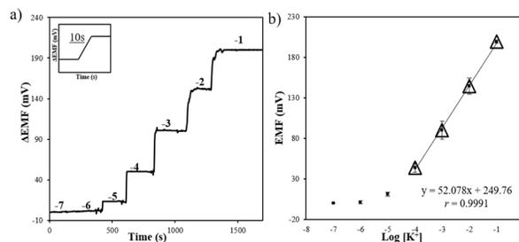
Fig. 3. Potentiometric response for three different PB-ISEs. In the left (a) is showed the time trace and in the right (b) the corresponding calibration plots after the addition of the potassium. A single addition of the analyte is shown in the inset on the plot (a) with the time response.
