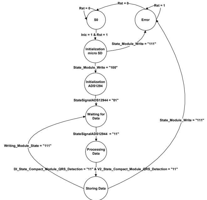
Fig. 3 General state machine (Note: When the signal Rst = 0 the next state is always S0, it was not included to better understand the diagram).
