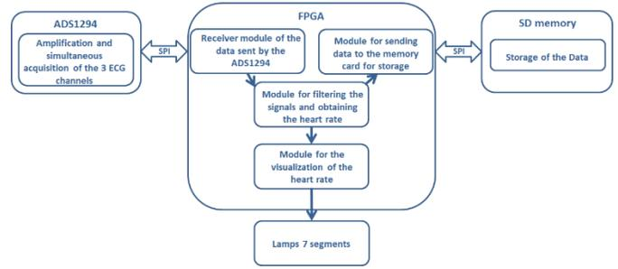
Fig. 2. Block diagram of the prototype of ambulatory ECG monitoring system of 3 leads with R wave detection in real time.
