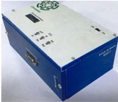
Fig. 4. Prototype of ambulatory ECG monitoring system of 3 leads with R wave detection in real time.
