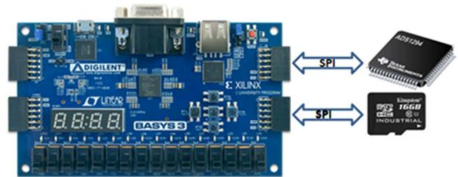
Fig. 1. Main components of the prototype of ambulatory ECG monitoring system of 3 leads with R wave detection in real time.
