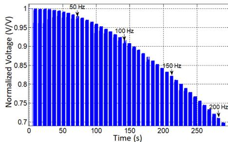
Fig. 5. Normalized output voltage of the prototype in the frequency range from 0 Hz to 200 Hz for the calculus of the bandwidth.
