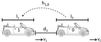
Fig. 2. Two connected vehicle systems under the CCC strategy.
