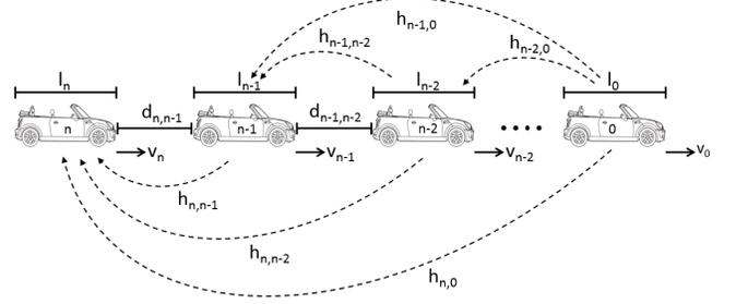
Fig. 1. Connected vehicle systems. The variables  $l$  and  $d$  are the length of the vehicle and the inter-vehicular distance, respectively. The variable  $h$  represent the time delay generated by signal transmission. Finally, the variable  $v$  is the velocity of the vehicle.
