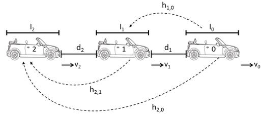
Fig. 7. Three connected vehicle systems under the CCC strategy.
