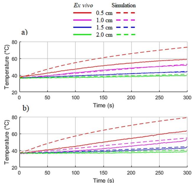
Fig. 4. Temperatures reached in the simulation and experimentation with 10 W input power and 5 min of radiation. a) MTM antenna and b) DSC antenna.
