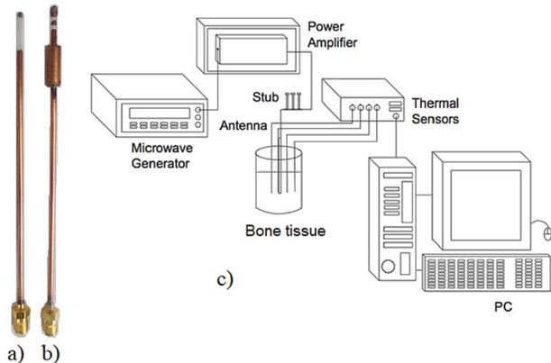
Fig. 2. MWA antennas and radiation system. a) MTM antenna. b) DSC antenna. c) radiation and thermometry system.
