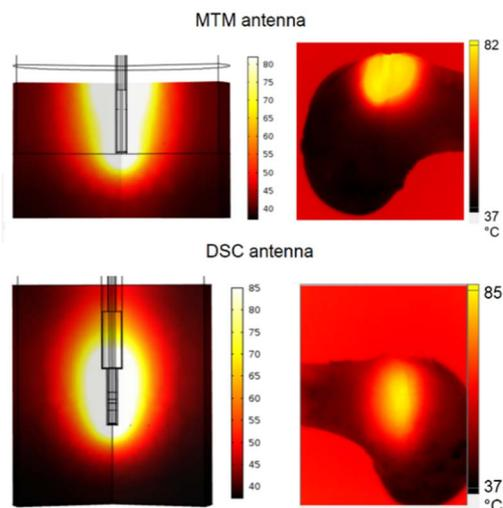
Fig. 5. Heating pattern generated in simulation (left) and experimentation (right) in bone tissue using MTM and DSC antennas.
