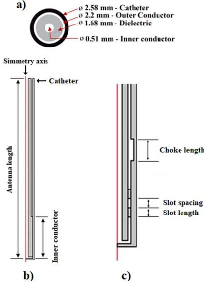
Fig. 1. Schematic design of the antennas. a) Dimensions of the coaxial cable, b) MTM antenna, c) DSC antenna.
