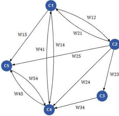
Fig. 1. Simple representation of an FCM
