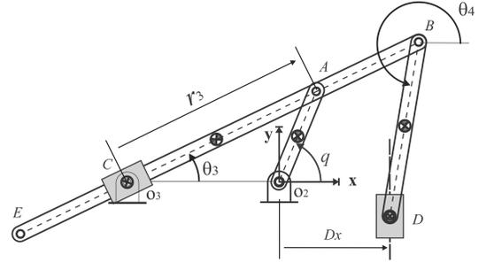
Fig. 1. Inverted Whitworth mechanism
