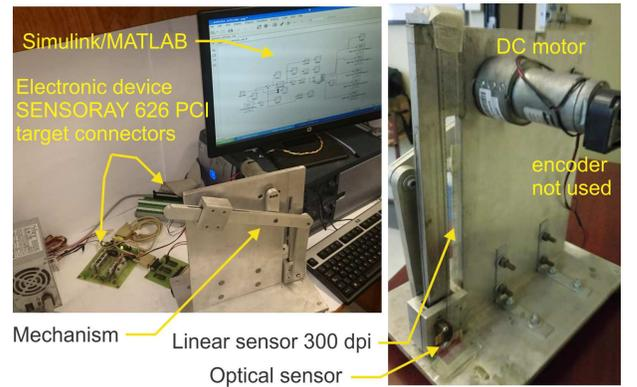
Fig. 2. Inverted Whitworth mechanism prototype
