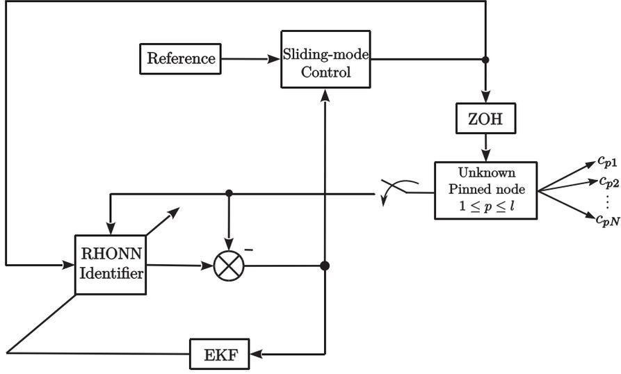
Fig. 1. Discrete-time neural sliding-mode pinning control scheme.
