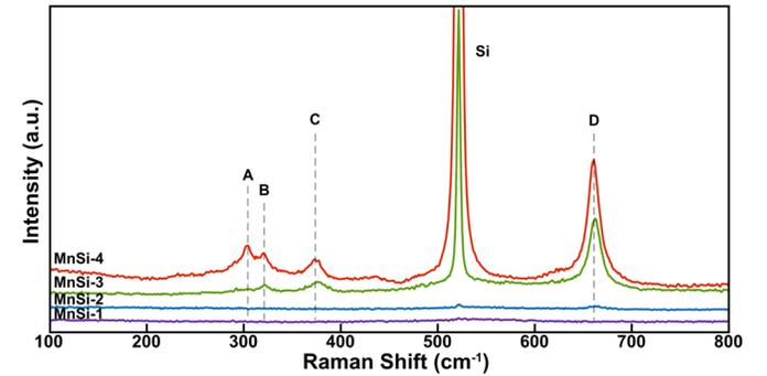
Fig. 4. Raman spectroscopy of the MnSi samples.
