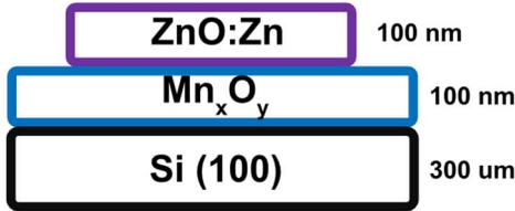
Fig. 2. Final structures with two layers, the first one of Mn with thermal oxidation and a ZnO:Zn as the last one. The samples are named ZnMnSi.
