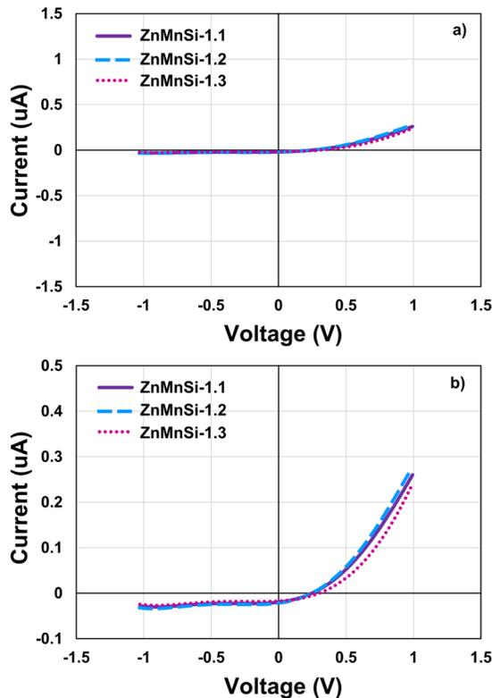
Fig 7. Current-voltage curves to test the reproducibility of the ZnMnSi-1 structure.
