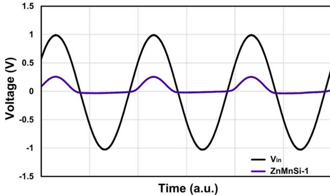
Fig. 6. The signal observed in the time domain for the ZnMnSi-1 structure.  $V_{in}$  is a sinusoidal signal of 100 Hz. The response is attenuated but the structure acts as a diode and the signal obtained is a typical half-wave rectifier.
