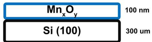
Fig. 1. Structure for the deposition of Mn samples named MnSi.
