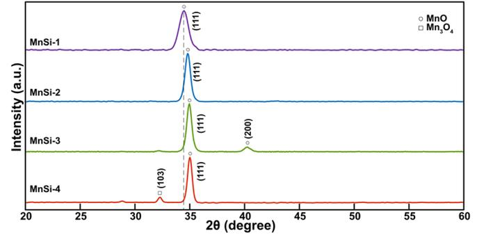
Fig. 3. X-ray diffraction patterns of the MnSi samples.
