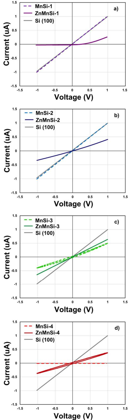
Fig. 5. Current-voltage transversal curves of the different structures.
