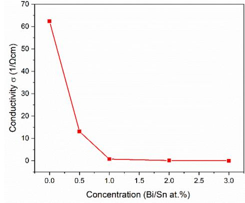
Fig. 3. Effect on electrical conductivity with respect to Bi/Sn concentration.
