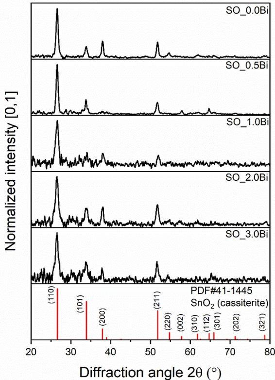
Fig. 1. XRD patterns of the SO\_X.XBi samples deposited at 400 °C.
