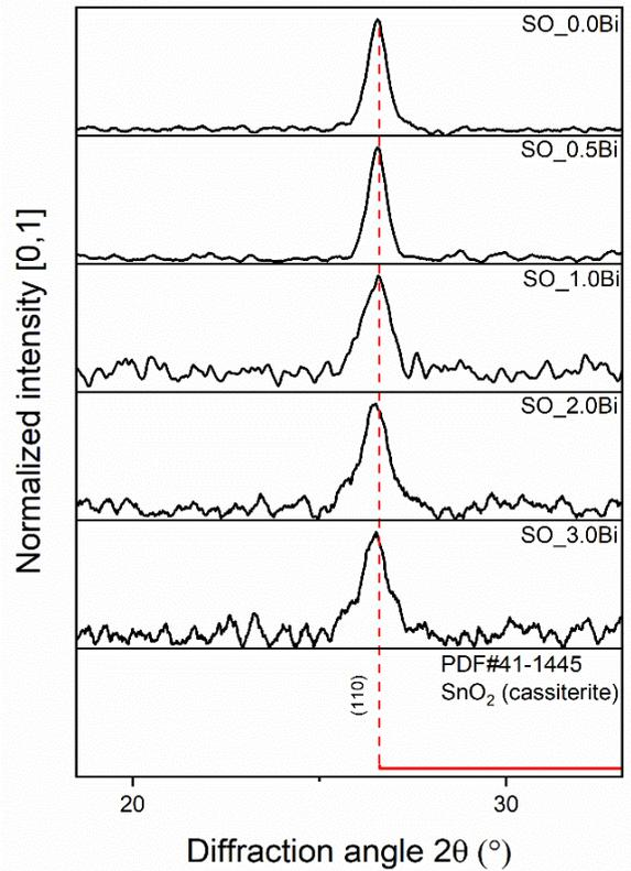
Fig. 2. Detail on the (110) plane region for the SO\_X.XBi samples from XRD patterns.
