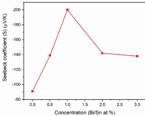
Fig. 4. Effect on the Seebeck coefficient with respect to the concentration of Bi/Sn.
